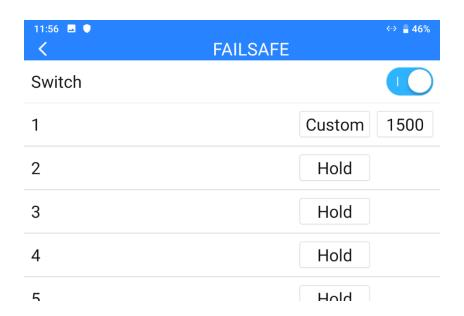
5. After configuration, the channel would output the value if the air unit lost communication with the ground unit during flight.
