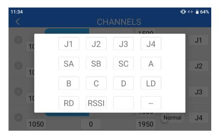
Select a target channel. Then touch a mapped button / switch / joystick, it will pop up a list of all physical channels. Select the button / switch / joystick you want to re-
