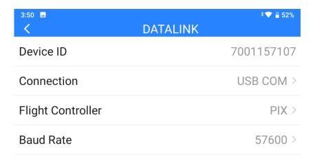
Run QGroundControl, go to "Application Settings – Comm Links" and "Add" a new connection. Name it as "USB-COM". Connection "Type" as "Serial". Match the baud rate.
